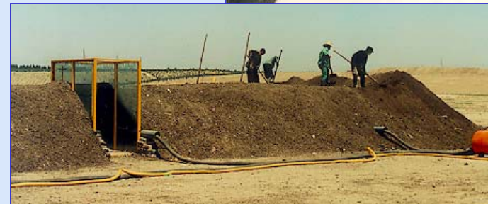
Example EuRec®-aerobe rotting process for 1.000 tons/d Tehran (Iran)
