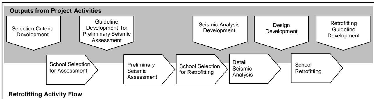
Fig2. Flow Chart of Retrofitting Process with Outputs
